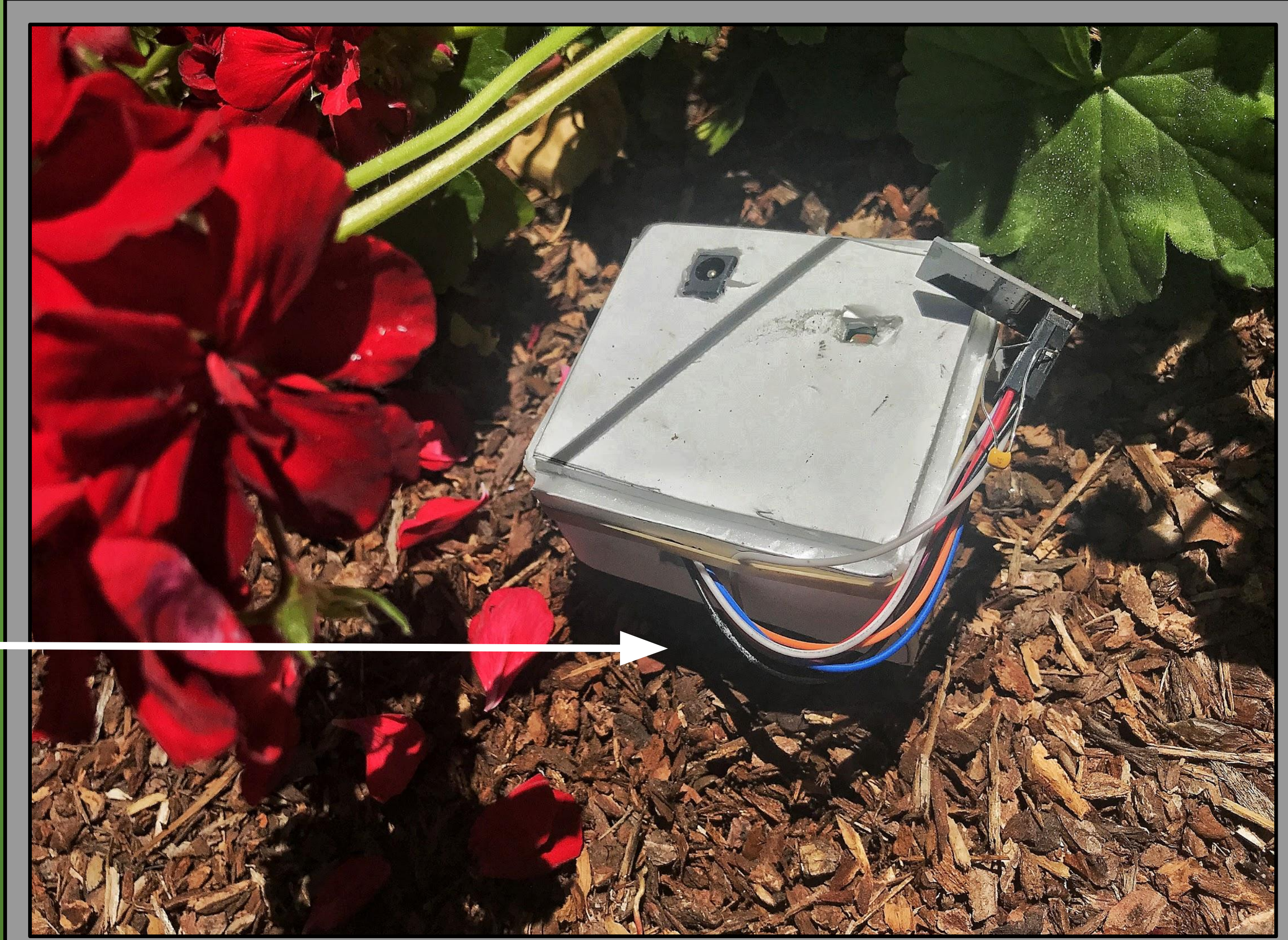
Figure 3: Sensor node with its protective covering placed in an ideal use-case location.
