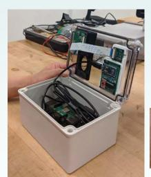
Preliminary prototype used to test sensors and algorithms used for line detection
