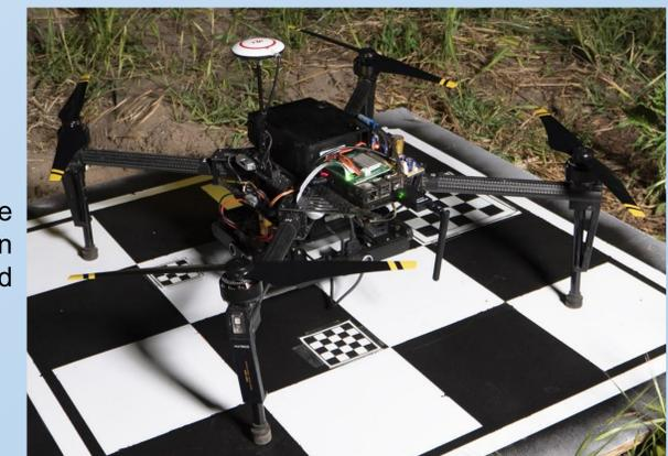
Our development drone with fire detection payload
